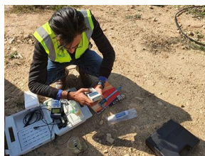
One of the trainees is measuring the salinity of water in the field
