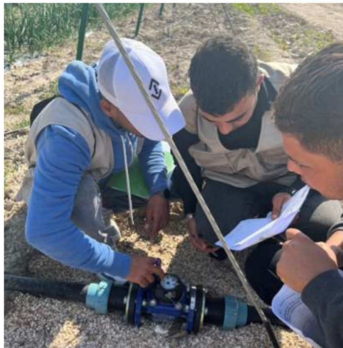
Youth participants take flowmeter reading to determine the applied irrigation depth during an irrigation event
