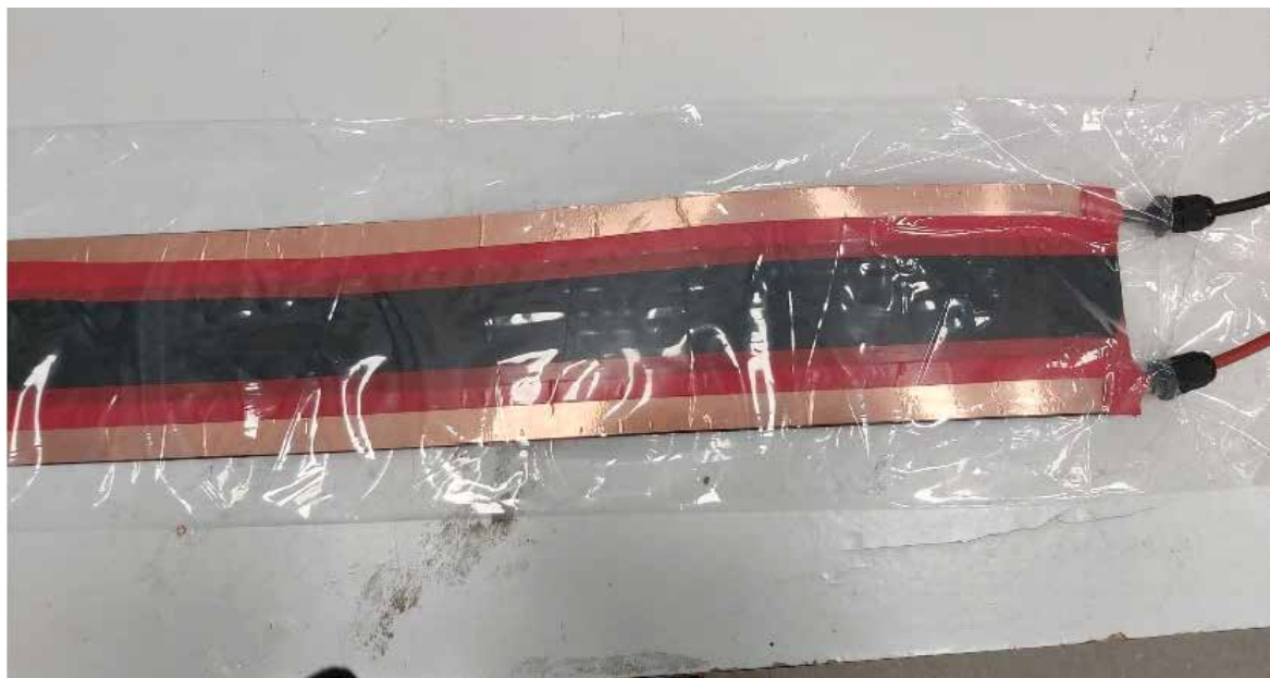
One of the AZMUD project technologies, the Joule Heating Conductive Plastic Sheets, used to heat the root-zone in soilless agriculture, a technology developed by AIMPLAS
