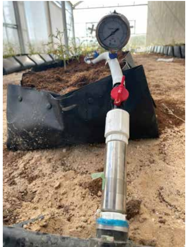
The Magnetic Water device, developed by NRC, Egypt, is being validated at MIRRA's Climate-smart Farm in the Jordan Valley
