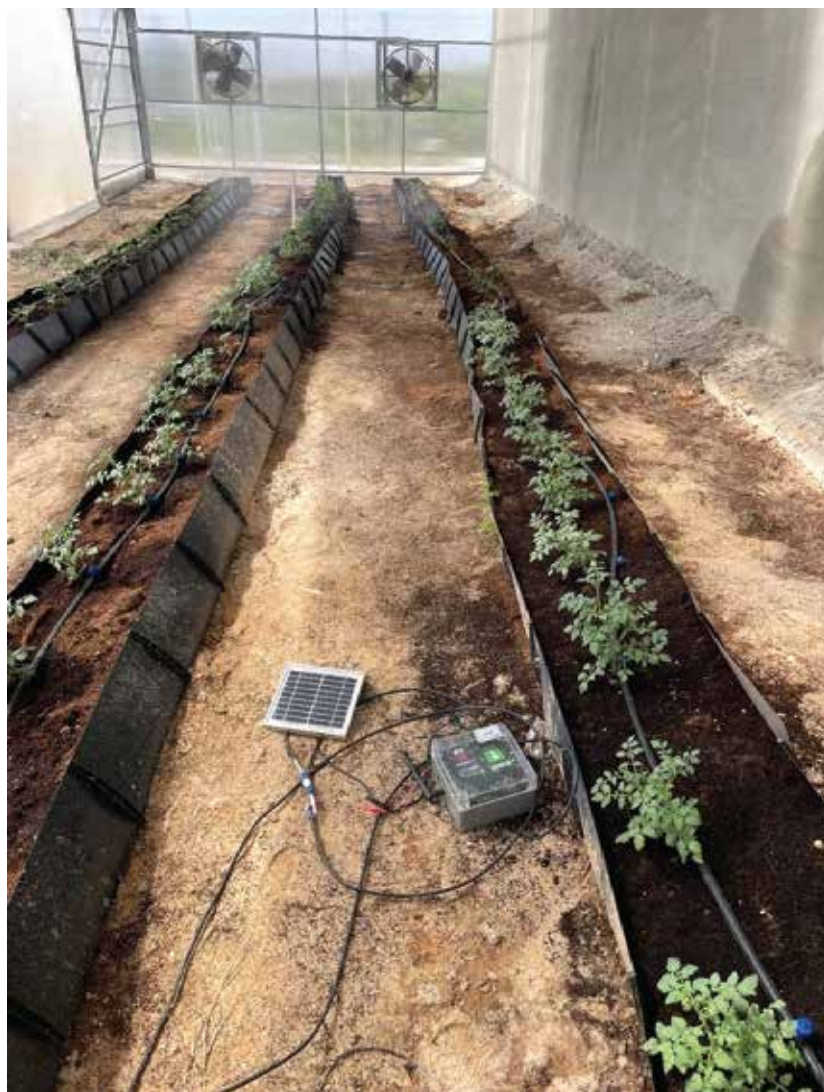
Low-energy Drip Irrigation Systems is Piloted in Jordan along with temperature and humidity sensors as part of the AZMUD project
